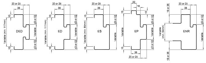
**Note:** When installed with appropriate door leaf, frames are fire rated up to 4 hours in masonry walls, and 2 hours in dry wall. Custom frame profiles available on request. Frames are typically 1.2-1.6 zincanneal unless otherwise requested.
